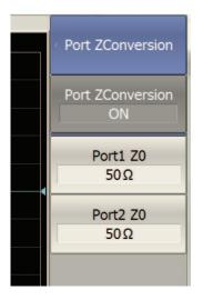
The function of conversion of the S-parameters measured at 50  $\Omega$  port into the values, which could be determined if measured at a test port with arbitrary impedance.
