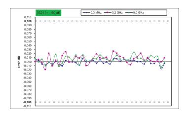
Low trace noise allows for particularly high-precision measurements. This graph shows the variation of the absolute value of the measurement error of  $S_{21}$  and  $S_{12}$  when the value of  $|S_{21}|$  and  $|S_{12}|$  is -50 dB, using 42 different Planar 804/1 VNAs. With the model's specificed accuracy of  $\pm$  0.1 dB, the trace clearly shows that the variation within the device pool is well below that figure. This confirms the precision of the instrument.
