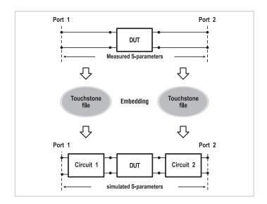
This function allows the user to mathematically simulate DUT parameters by virtually integrating a fixture circuit between the calibration plane and the DUT. This circuit should be described by an S-parameter matrix in a Touchstone file.
