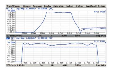
Limit testing is a function of automatic pass/fail judgment for the trace of the measurement results. The judgment is based on the comparison of the trace to the limit line set by the user and can consist of one or several segments.
