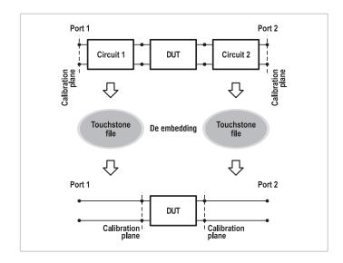
This function allows the user to mathematically exclude the effect of the fixture circuit connected between the calibration plane and the DUT from the measurement results. This circuit should be described by an S-parameter matrix in a Touchstone file.
