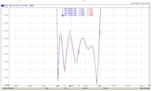
System VSWR across 20 MHz using New Calibration Method
