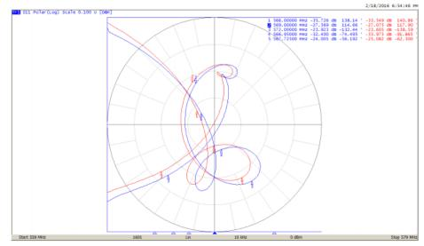
Polar Display of System Impedance across 20 MHz using New Calibration Method
