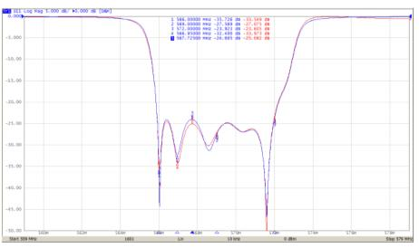
System Return Loss across 20 MHz using New Calibration Method
