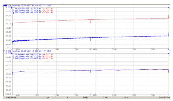
In both 21 plots, the red trace is the coupling reference, and the blue trace is the reverse measurement. The difference between the traces is the directivity.
