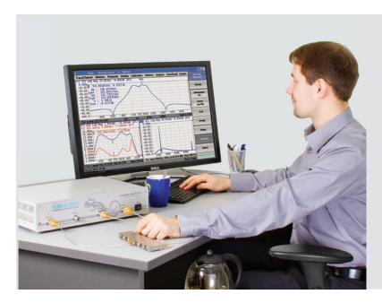
The Planar 808/1 VNA is an S-parameter vector network analyzer designed for operation with an external PC. It connects to any Windows-based computer via USB and delivers accurate testing and measurement through a platform that reduces points of data transfer and keeps up with advancing technology.
