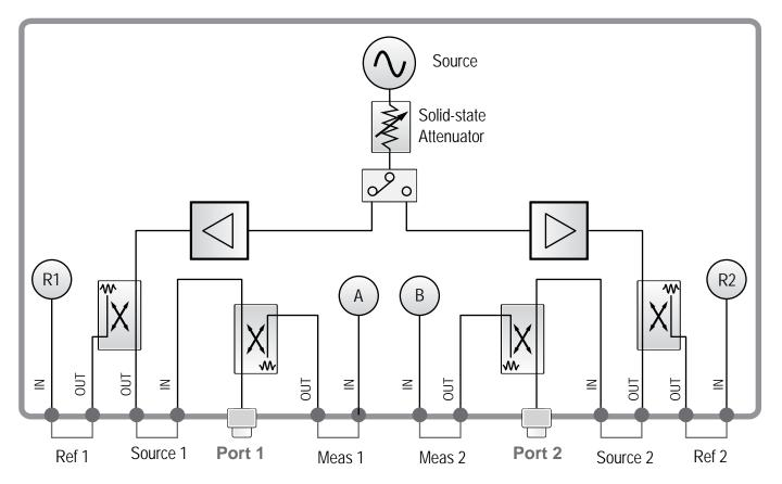
This 2-port analyzer offers adjustable port configuration with direct access to the receivers.
