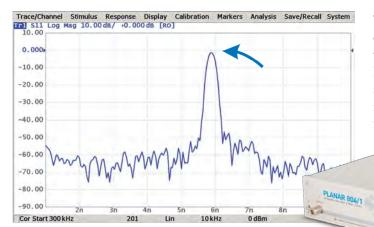
This function performs data transformation from frequency domain into response of the DUT to various stimulus types in time domain. Modeled stimulus types: bandpass, lowpass impulse, and lowpass step. Time domain span is set by the user arbitrarily from zero to maximum, which is determined by the frequency step. Windows of various forms are used for better tradeoff between resolution and level of spurious sidelobes.
