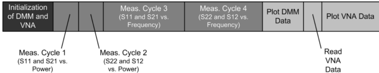
Figure 3: During the first sweep cycle, Port 1 generates a Power Sweep signal while the VNA measures S_{11} and S_{21} . Next, the generator switches to Port 2 and a reverse Power Sweep is performed, allowing the VNA to measure S_{22} and S_{12} . Frequency Sweeps from Port 1 and Port 2 are the 3rd and 4th sweeps respectively.
