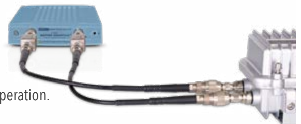
Pictured here is an SC5090 VNA testing a 75 \Omega amplifier with two CMT AP50NM75NF Impedance Matching Pads.
