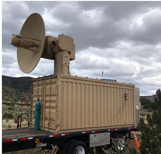
Verus Research designed the antenna for the Air Force Research Lab's Tactical High-Power Operational Responder (THOR) system (pictured above). Verus Research utilized CMT's VNA products for calibration and measurements of components leading up to the final assembly.
