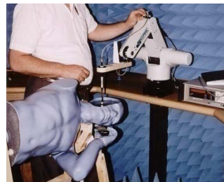
Near Field Probe and human torso phantom for measuring SAR
