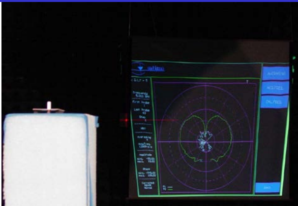
Real time 2D elevation pattern projection of a monopole antenna, on the wall of one of the Stargate-64 chambers used by CIA March 19, 2021
